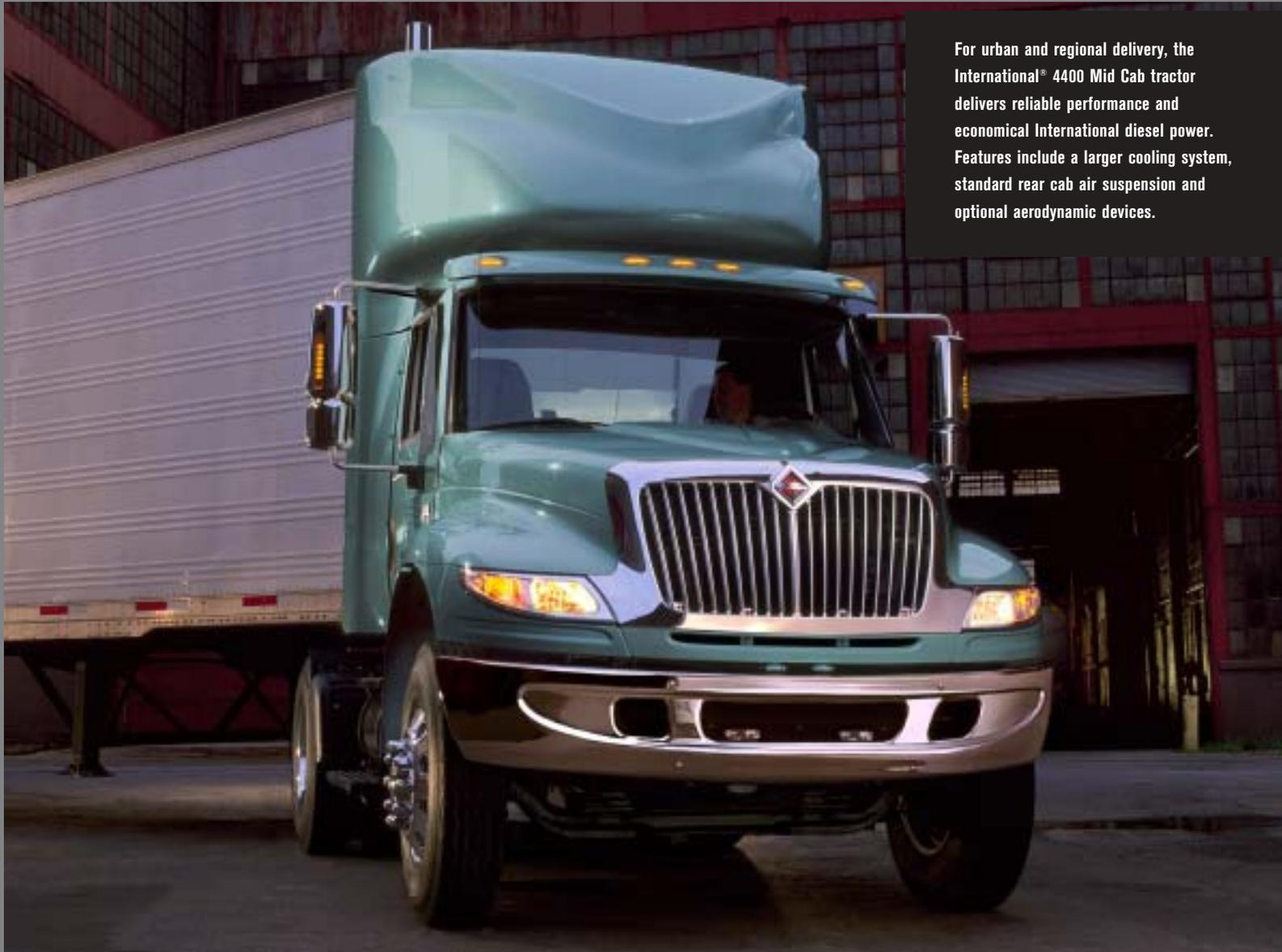
For urban and regional delivery, the International® 4400 Mid Cab tractor delivers reliable performance and economical International diesel power. Features include a larger cooling system, standard rear cab air suspension and optional aerodynamic devices.
