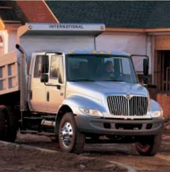
The optional crew cab (above) accommodates up to six passengers and features a four-door design with well-placed offset steps and a three-point entry system for easy entry and egress. Standard rear cab air suspension provides an extraordinarily smooth ride and longer cab life. Wide rear cab doors open a full 85°.
