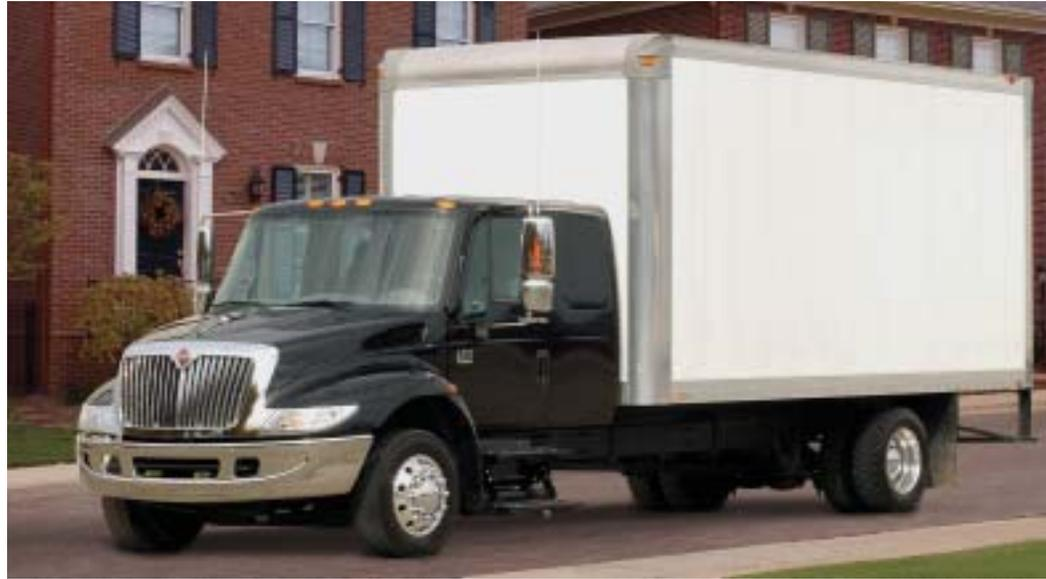
The International® cab is the industry's most spacious, quiet and comfortable. And the most durable – with one-piece door frames, double-sided galvanized steel construction and a three-step E-Coat prime/base coat/urethane clear coat paint process.
